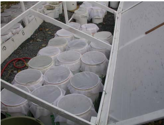
Figure 3. The microplots at Maritime MicroBiologicals Inc. The roof that keeps rain off the plots facilitating moisture control, is in the open position. Fine mesh is over the plots.
